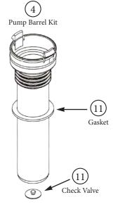
Parts Kit Includes: Spring Plunger Cup Assembly Grease Pack Viton® Diaphragm Check Valve Viton\* Diaphragm
