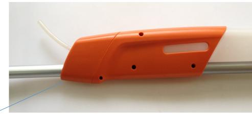
Unscrew 6 screws on body, 4 screws on front, one in bottom and last one inside.
